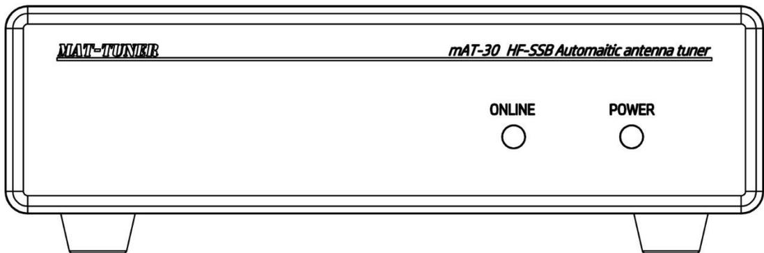
**ONLINE:** Tuner is Active or Bypass. Lights up to indicate that the tuner is online, off indicates that the tuner is in bypass.
