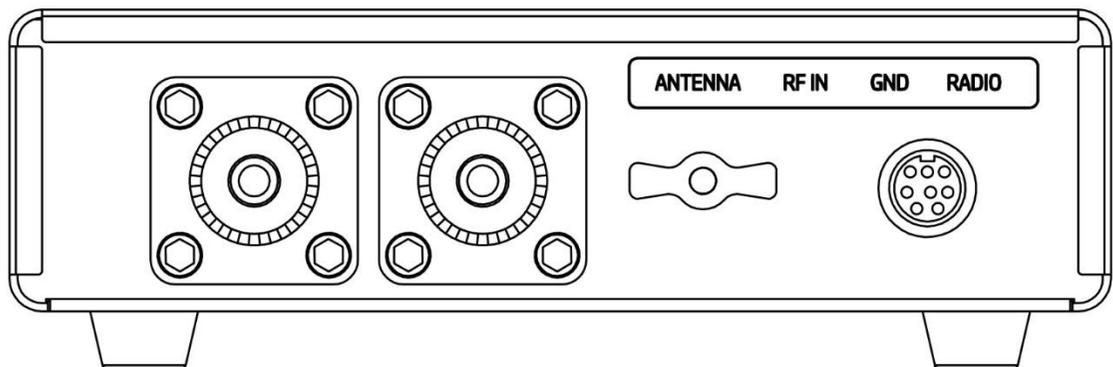
**ANTENNA:** SO-239, this socket is connected to the antenna via 50 ohm coaxial cable.
